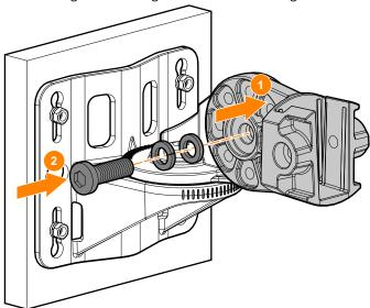
8. Slide the holder of the AP into the opening of the mounting holder and use two M6x20 screws (included in the package) to fix the AP to the mounting holder as shown in Figure 6. We recommend to torque the M6x20 screws to 2.5 N.m.
