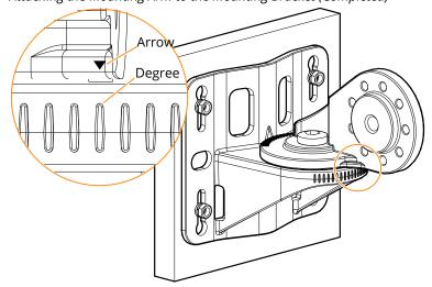
7. Use the M10x30 screw (with washers) included in the package to fasten the mounting holder to the mounting arm as shown in Figure 5. We recommend to torque the M10x30 screw to 12 N.m.
