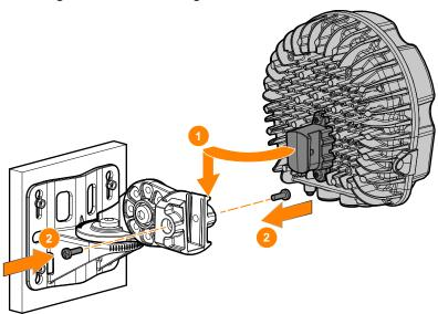
9. The vertical angle of the AP can be adjusted +/-45 degrees by inserting an M6x20 screw (included in the package) into the different holes on the mounting holder as shown in Figure 7. We recommend to torque the M6x20 screw to 2.5 N.m.
