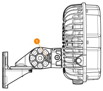
10. Use the cable tie to fasten the cables on the mount kit.
