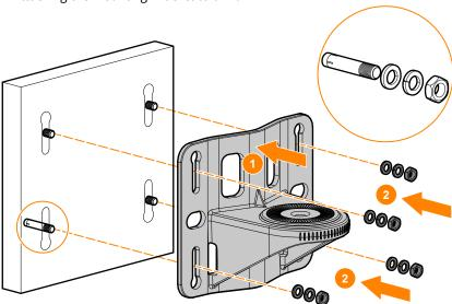
6. Place the mounting arm in your desired horizontal angle by aligning the arrow marking on the mounting arm to the appropriate degree marking on the mounting bracket. The horizontal angles of the AP (mounted on the AP-270-MNT-H3 mount kit) can be adjusted +/-45 degrees. Use the M10x30 screw (with washers) included in the package to attach the mounting arm to the mounting bracket as shown in Figure 3 and Figure 4. We recommend to torque the M10x30 screw to 12 N.m.
