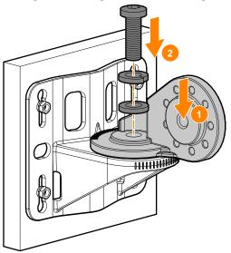
**Figure 4** Attaching the Mounting Arm to the Mounting Bracket (Completed)
