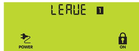
When exit time has expired, the keypad will display that the home area (Area 1 in this case) is on, and that area 2 is also on via the area icons.
