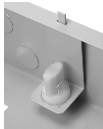
Figure 2: Tamper Bracket Installation
