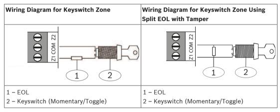
Tab. 13.20: Wiring Diagram for Keyswitch Zone
