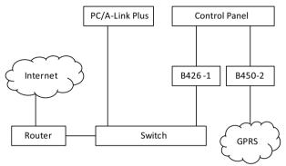
In the configuration diagram above, the control panel is programmed with Transmission Format as Email and two network modules are enabled to access mail server. It is an example of using B426/B426-M as network module 1 and B450/B450-M as network module 2. The wiring diagram is shown in above picture. "B426-1" means the rotary address switch of B426-M is set to 1; "B450-2" means the rotary address switch of B450-M is set to 2.
