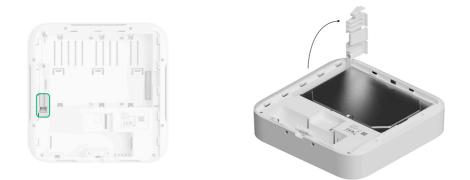
**4.** Install the hard drive in the NVR enclosure so that the connectors match.
