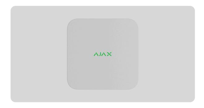
**NVR** is a network video recorder for home and office video surveillance. You can connect **Ajax cameras** and third-party IP cameras to the device.
