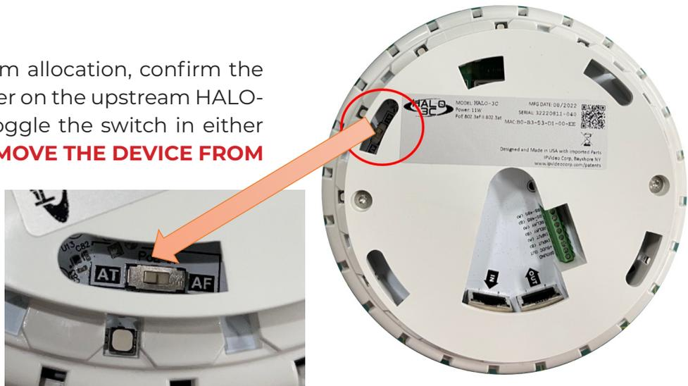
With the upstream HALO-3C in AT power mode, you can connect an ethernet cable from the output RJ45 into an 802.3 af PoE device.
