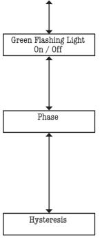
Green flashing light on / off. By using the right and left keys you can turn the green flashing LED, located on the head and controller, on or off. This is a useful way of identifying the beam head you are working with (press enter to return to mode change or down to go to phase).
